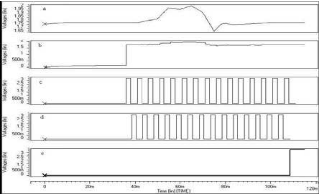
Fig. 8. (a) Input to S/H circuit. (b) Sampling signal of the 1st stage. (c) CK1. (d) CK2. (e) CK3. In Fig. 8, the input rhythm of ST is applied to the S/H circuit and output of 1 st stage is shown.
