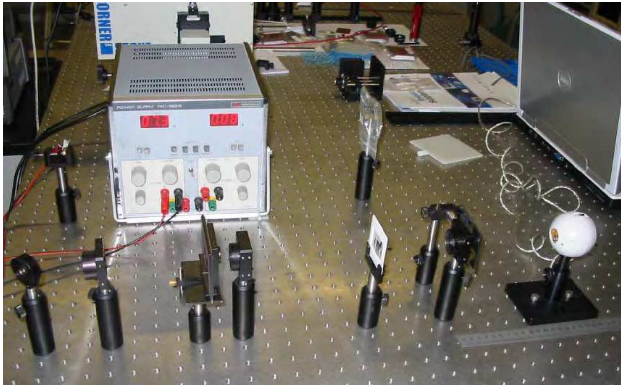
Fig. 9. CGH experimental setup
