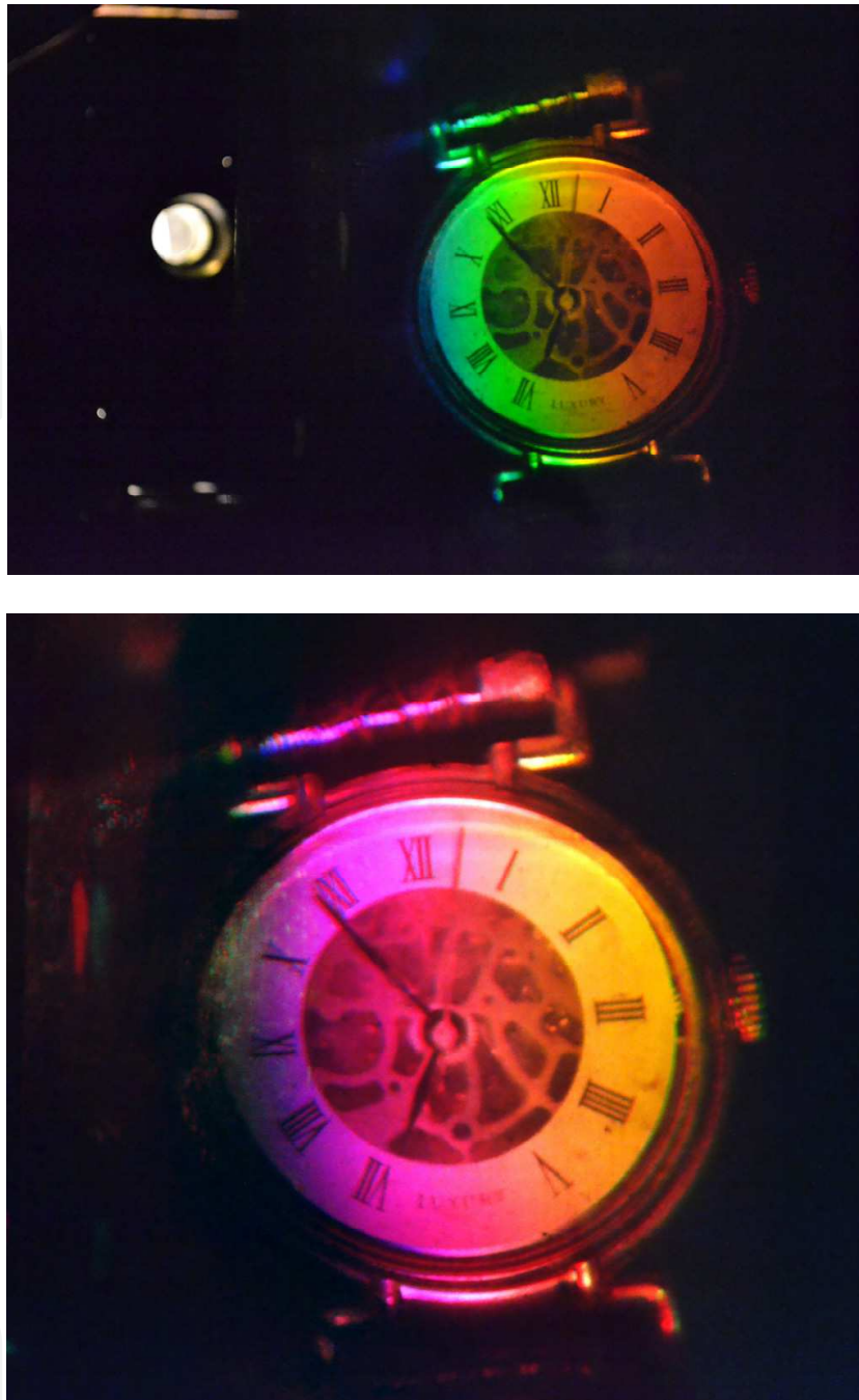
Fig. 4. Up: Photograph of an object directly projected on a holographic screen. Above: anaglyphic stereo representation of the same scene, with color channel.
