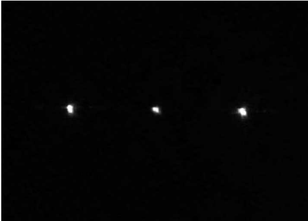
Fig. 8. Diffraction pattern captured with a CCD camera when addressing a binary grating with an averaged phase difference of 180 degrees.
