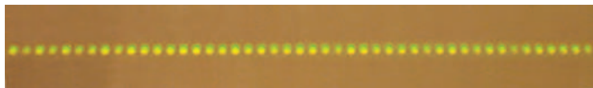
Fig. 11. Photograph of single parallax master-hologram. Each "shining" holopixel represents one view of the object.
