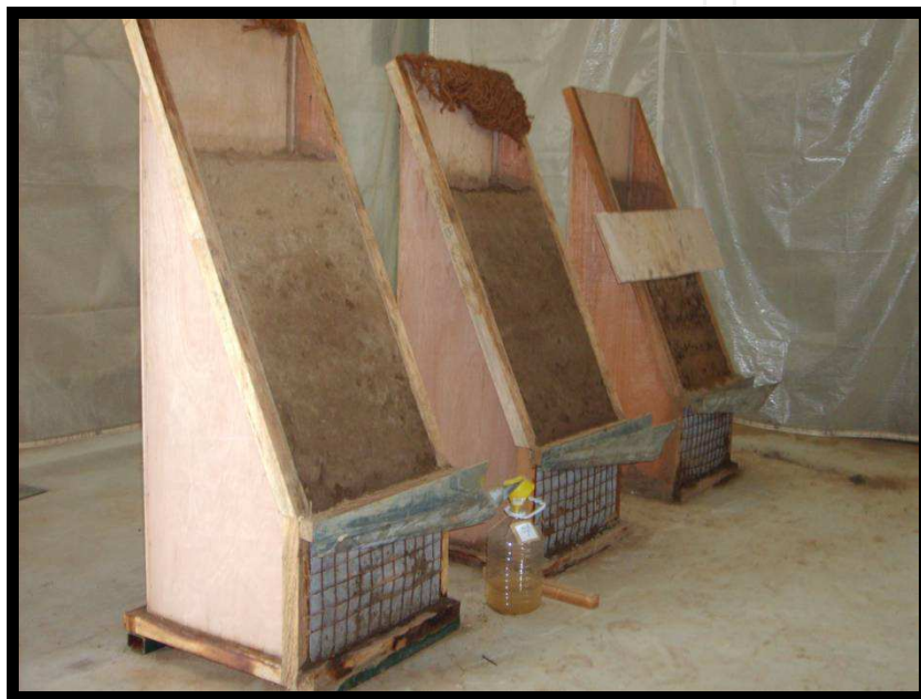
Fig. 2. Test boxes shown with compacted soil.
