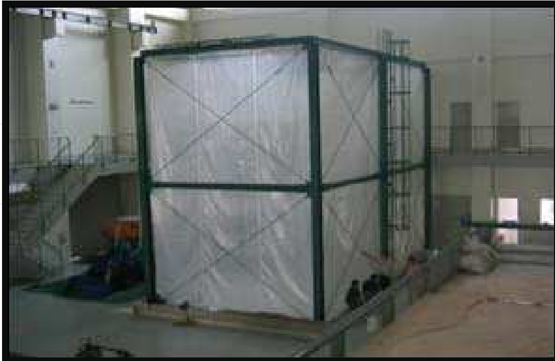
Fig. 6. Artificial Rainfall Simulation Apparatus at the Hydraulic Laboratory of the Flood Control and Sabo Engineering Center (FCSEC) of the Department of Public Works and Highways (DPWH).
