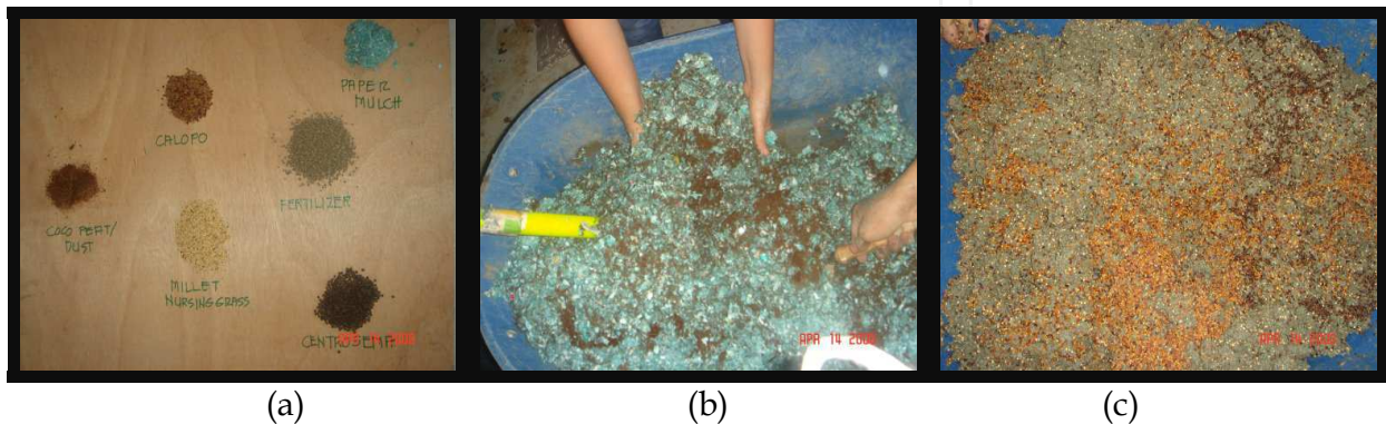
Fig. 3. The hydroseeding components and mixture. (a)Hydroseeding Mix Components(b) Mixing the components(c) Hydroseeding Mixture
