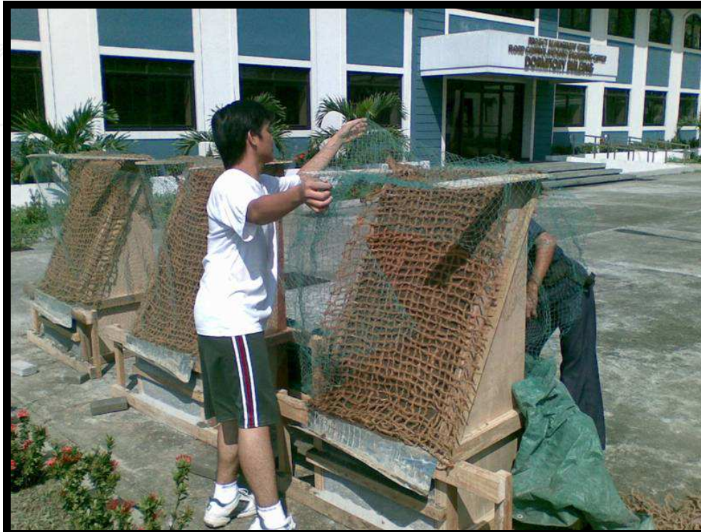
Fig. 5. Hydroseeded test boxes covered with coconet. The green net is used for protection from birds and other factors.
