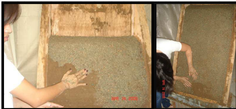
Fig. 4. Hydroseeding by manual application
