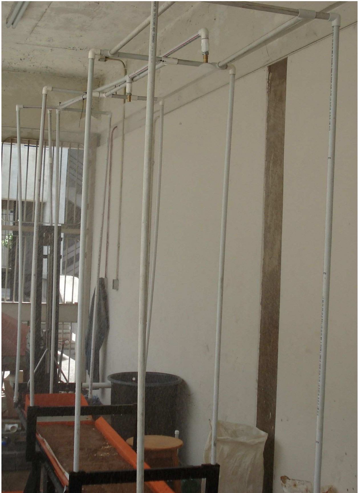
Fig. 2. The rainfall simulator with the soil bed
