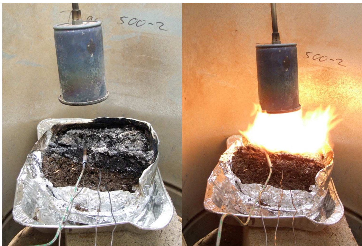
Fig. 8. Soil blocks were burned with a blowlamp reaching 250°C at 1 cm soil depth.
