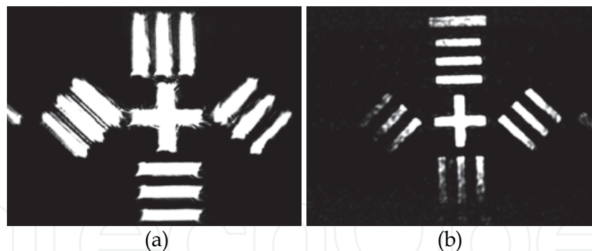
Fig. 26. Reconstructed images of (a) reference beam reconstruction hologram (Phase aberration image) and (b) conjugated beam reconstruction hologram (Corrected image)
