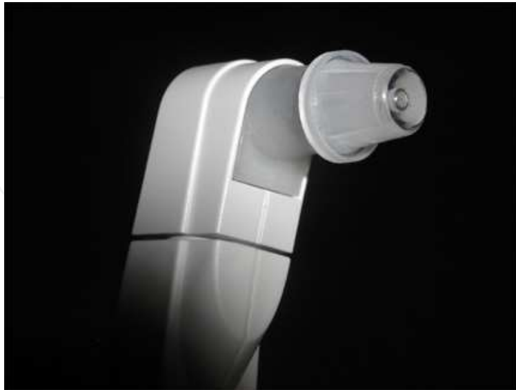
Fig. 10. The PASCAL® contoured piezoresistive sensor tip
