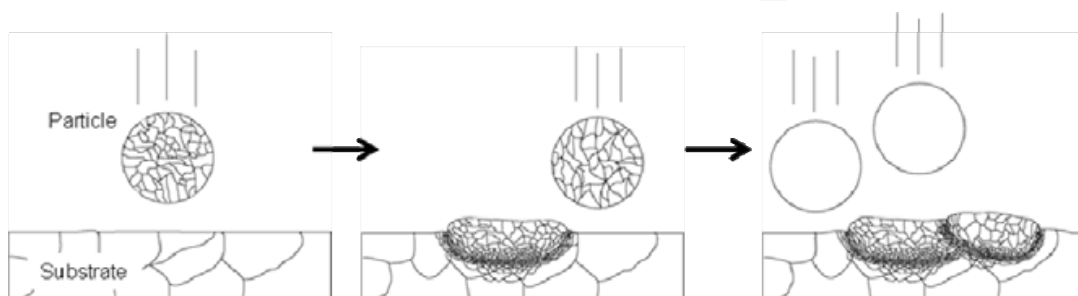
Fig. 28. Schematic of the powder grain changes by cold spraying
