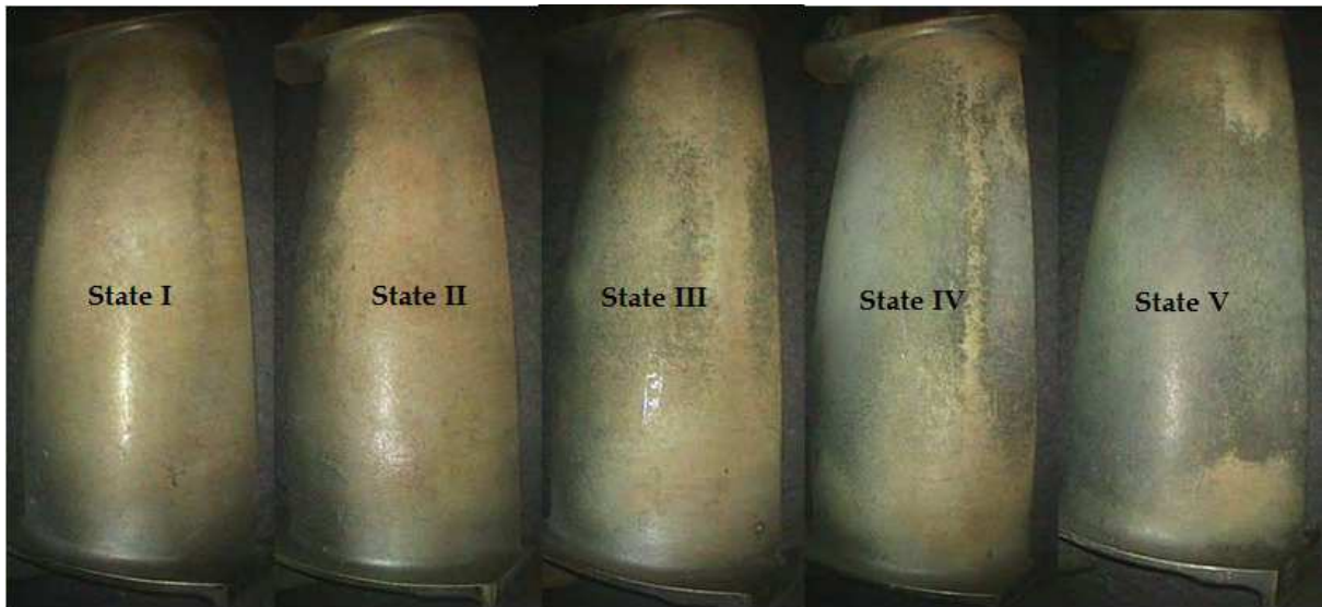
Fig. 17. Recording of vane surface images with a videoscope No. 2
