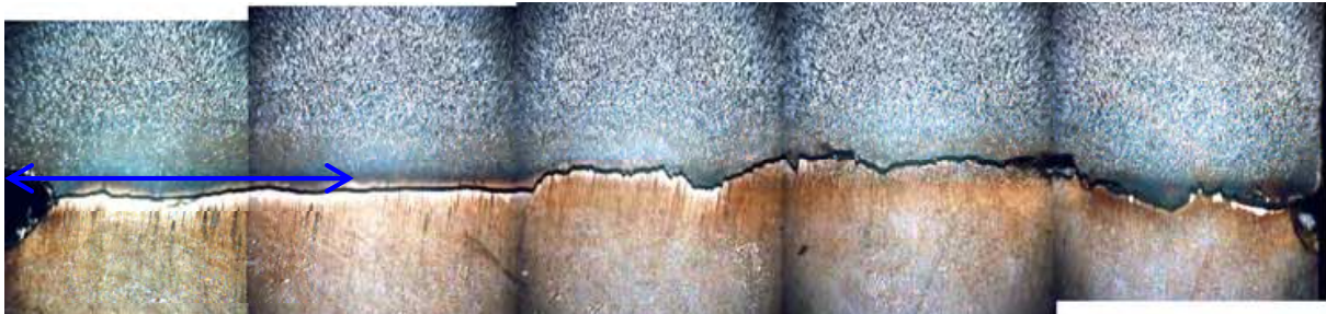
Fig. 23. Crack path for fracture toughness specimen corresponding to K_{Ic} = 15 MPa.m 1/2 .
