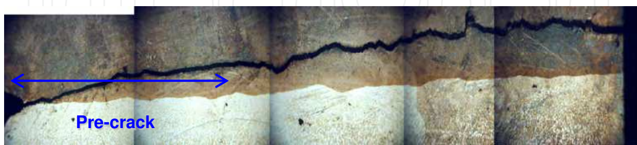
Fig. 24. Crack path for fracture toughness specimen corresponding to K_{Ic} = 45 MPa.m 1/2 .
