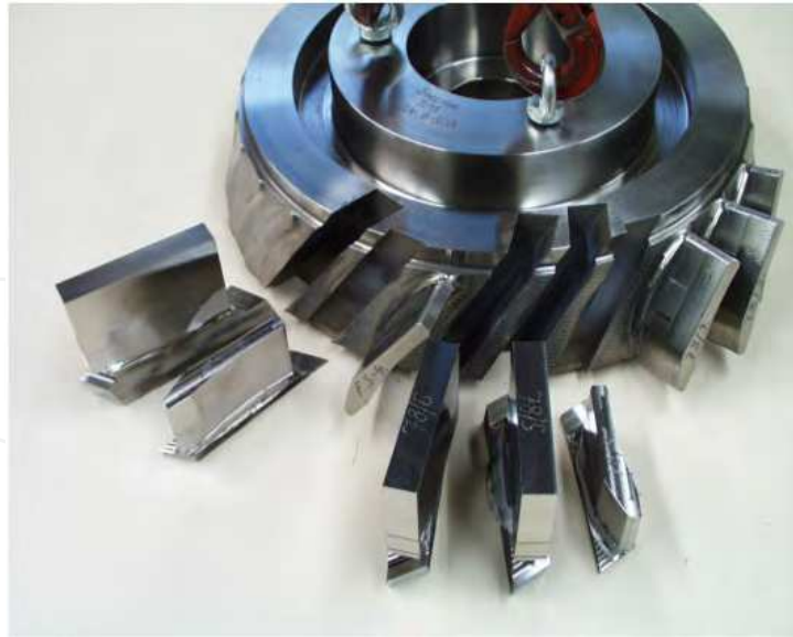
Fig. 26. Pre-machined BLISK demonstrator, after extraction of blade-blocks.
