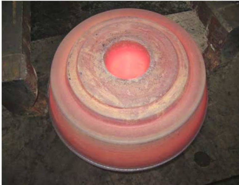
Fig. 8. Ti-6246 die-forged disk in the as-forged condition (courtesy by BSTG )
