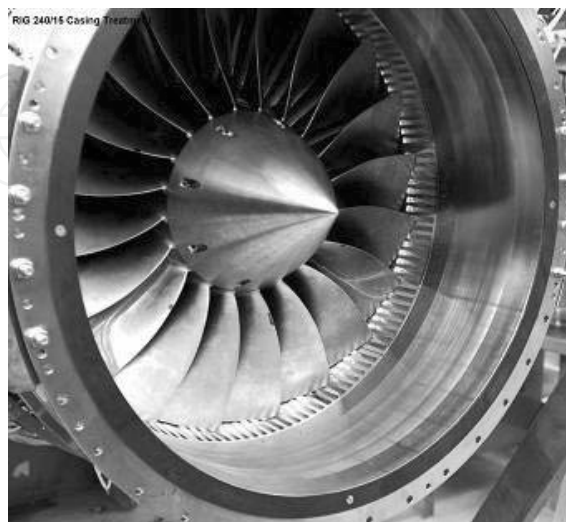
Fig. 12. EJ200 LPC with axial slots casing treatment (Broichhausen & Ziegler, 2005)
