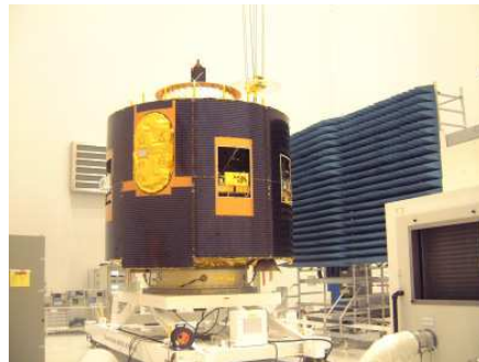
Fig. 17. Solar Array for spinning Satellite, Meteosat Second Generation (Credits: ESA - MSG Team)
