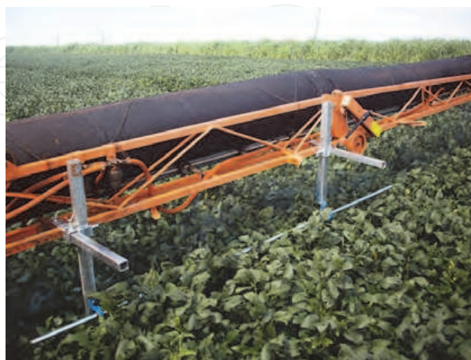
Fig. 5. Canopy opener artefact fixed to the spray boom in a soybean crop.
