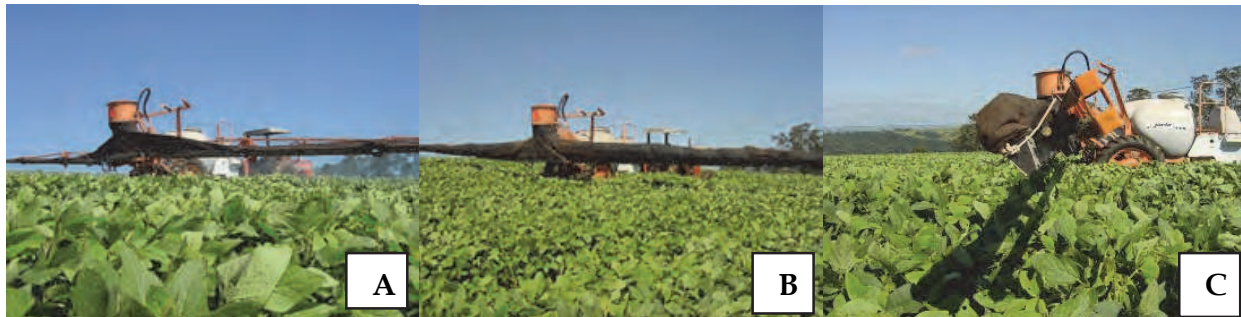
Fig. 3. Air-assisted sleeve boom sprayer in the following operation modes: A – conventional spraying (without air); B – spraying with air assistance at 0^\circ (vertical) and C – spraying with air assistance angled at 30^\circ forward to the displacement of the tractor-sprayer assembly on soybean crop.
