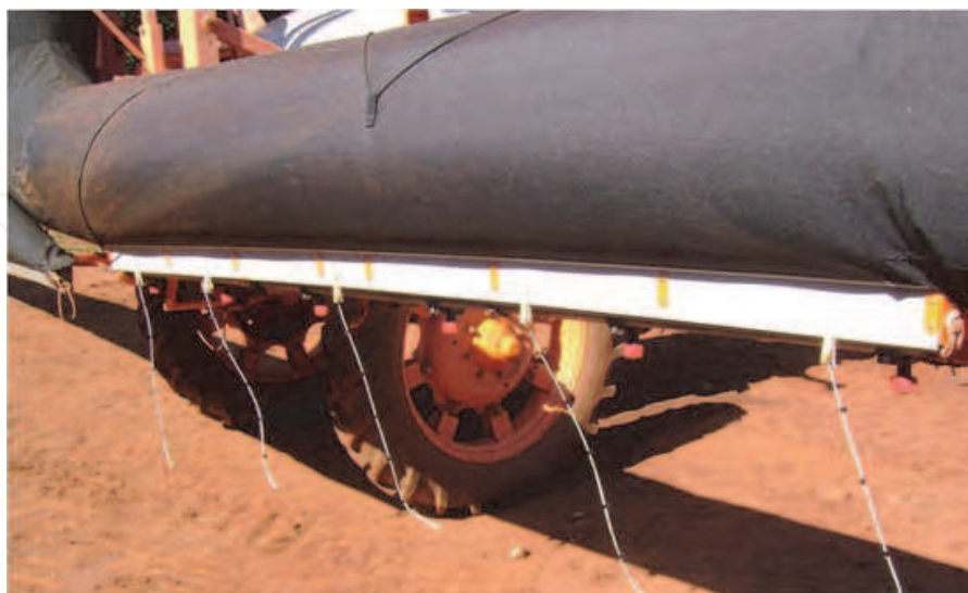
Fig. 1. "Nylon thread method" for measuring air speed in a sleeve boom sprayer.
