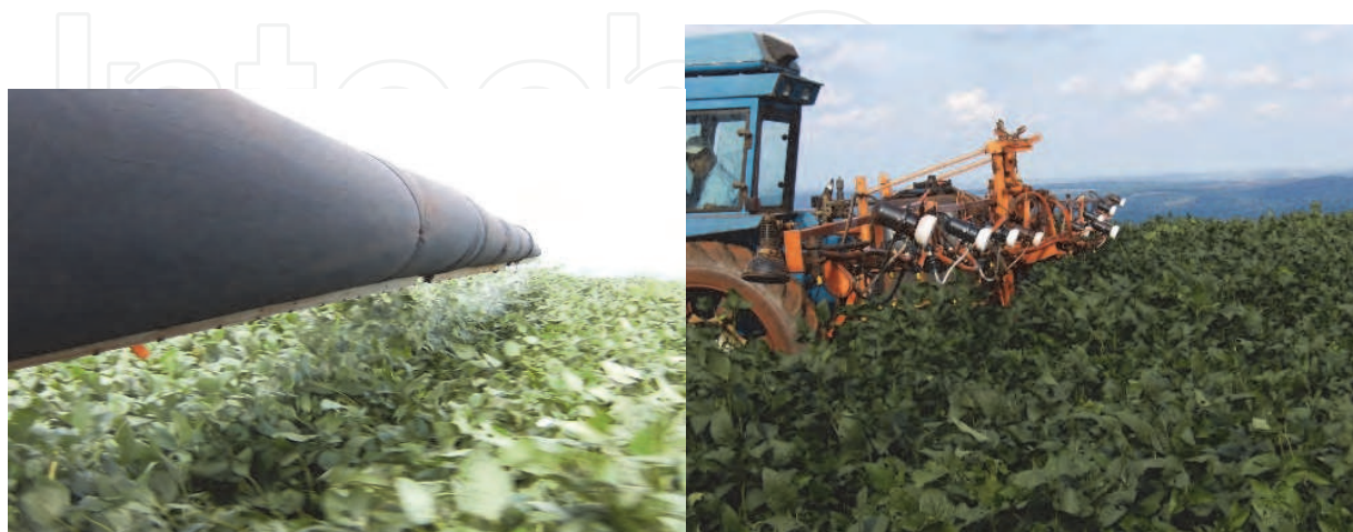
Fig. 7. Spraying with an air-assisted sprayer and rotating system nozzles fixed at the spray boom on soybean culture.
