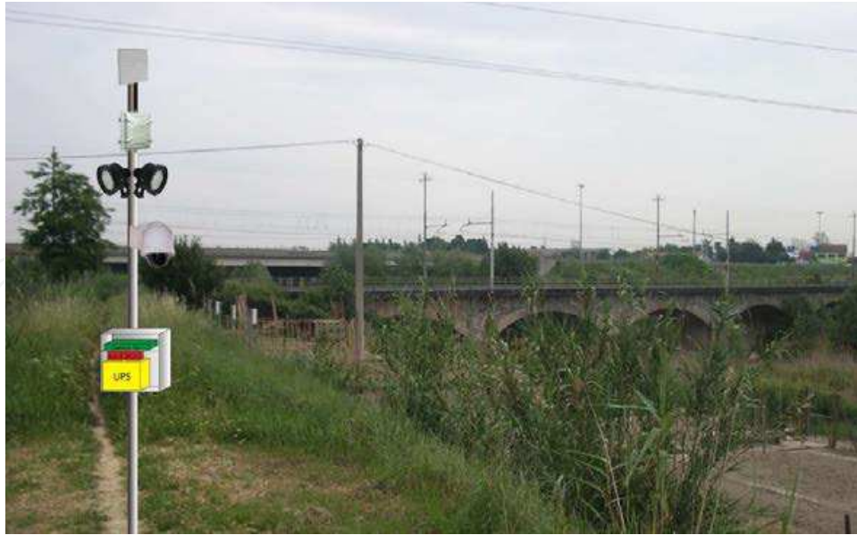
Fig. 11. Design of camera installation at the railways bridge over the “Savio” river, near “Cesena” city.
