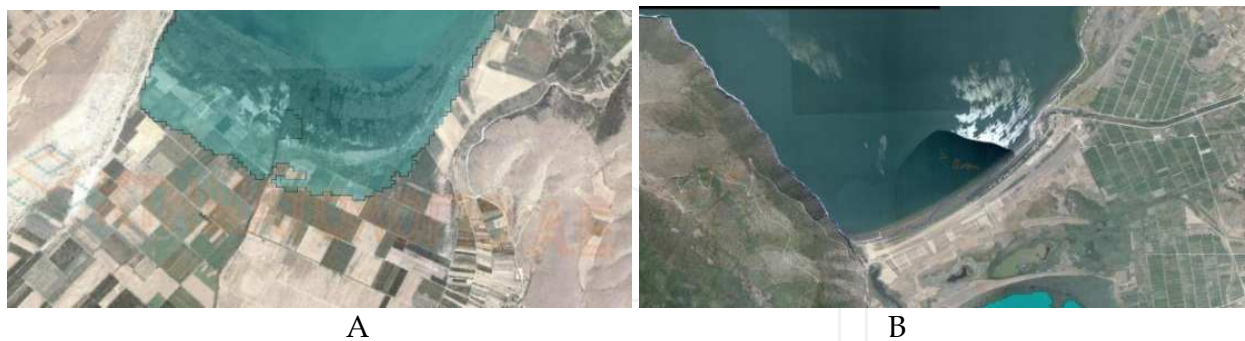
Fig. 8. Overlay of the coastlines extracted from the 17 th January 2011 image to the orthophoto of 0.5 m resolution A. south part of Vegoritiss lake B. South part of Macro Prespa lake.
