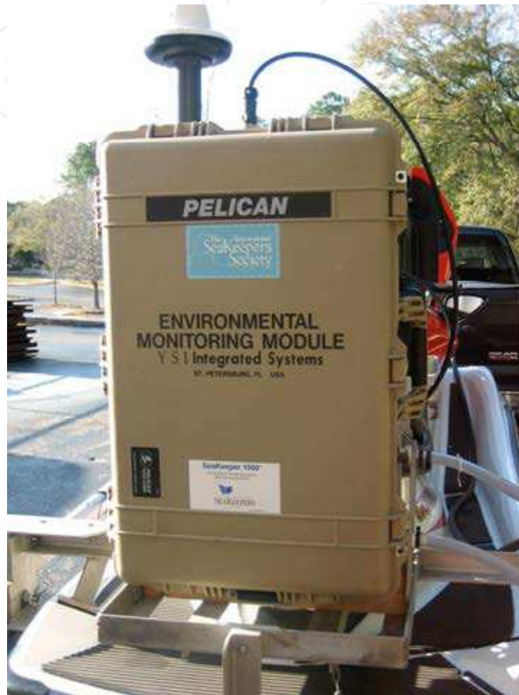
Fig. 5. The YSI Portable SeaKeeper 1500 mounted on the stern of the Jag Ski.
