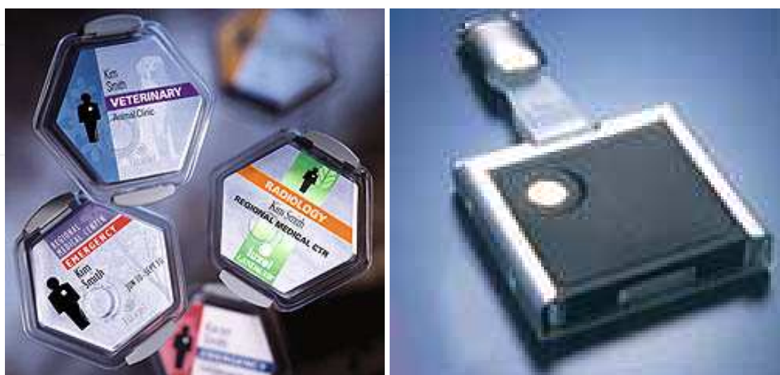
Fig. 7. Photographs of the OSL dosimeter (Type S) as shown the left photo picture and of the DIS dosimeter (Type DIS-1) as shown in the right photo picture.
