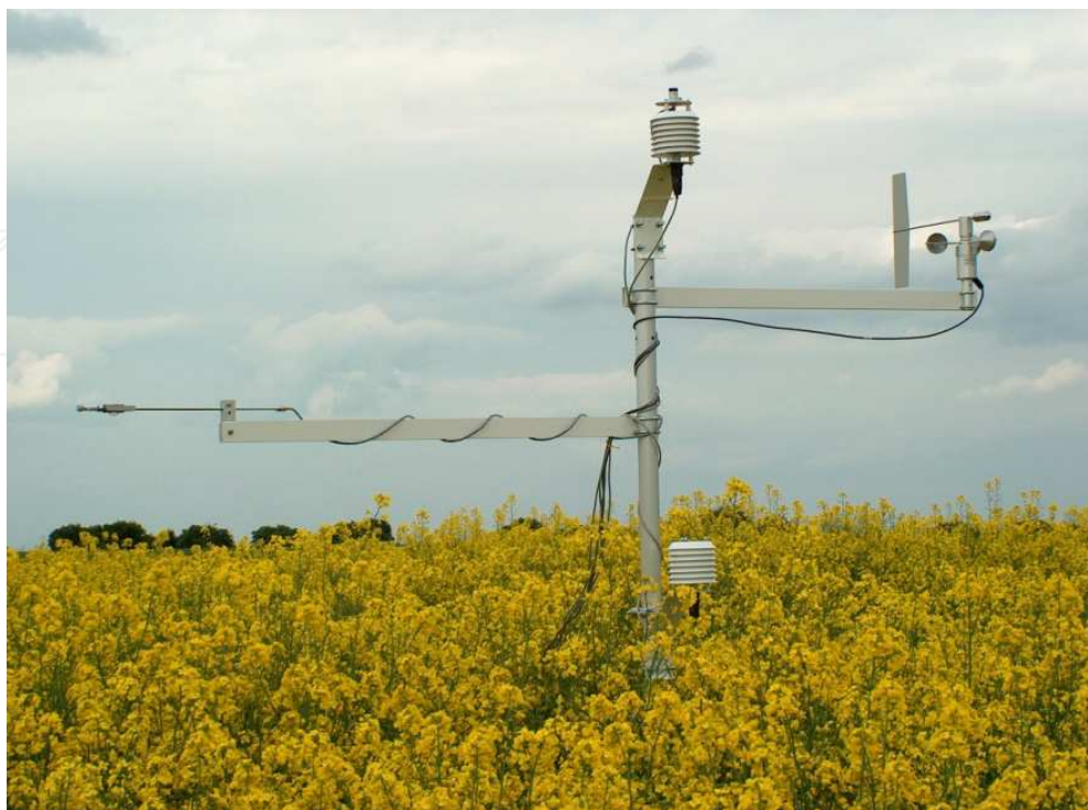
Fig. 1. BREB installation over winter rape-seed field: radiation balance gauge on left, pair of temperature/relative humidity sensor in the middle (upper with global radiance gauge), anemo-indicator on right. Locality: Červený Újezd 2006, photo by authors.
