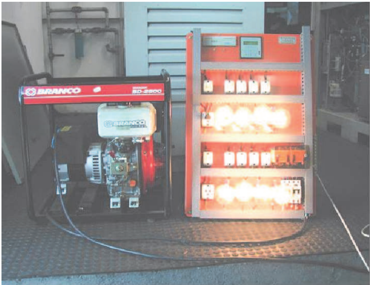
Fig. 1. Stationary engine and control panel (operating).
