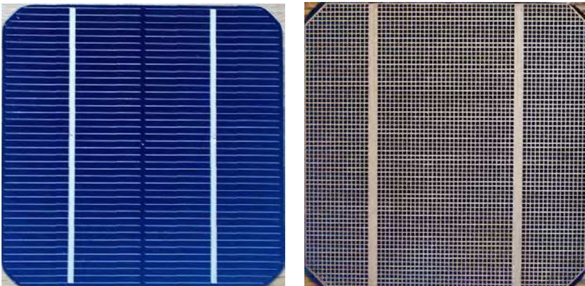
Fig. 5. Front and back side of monocrystalline silicon solar cell.
