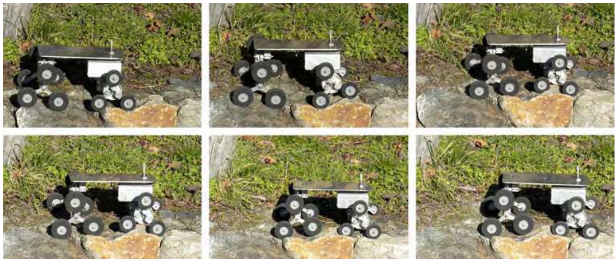
Fig. 12. Epi.q-1 in advancing mode, on uneven ground
