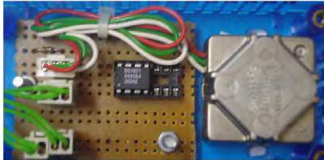
Fig. 23. Gyroscope with microcontroller worked on I 2 C bus as slave
