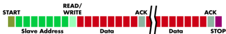
Fig. 16. The I 2 C bus communication
