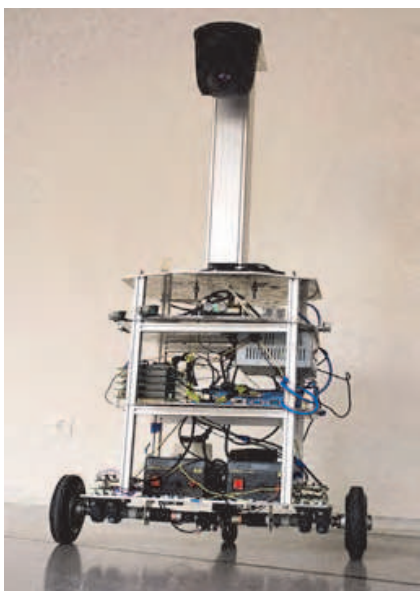
Fig. 2. (a) The open mobile educational platform PRIM. (b) Sensorial and electronic system blocks.
