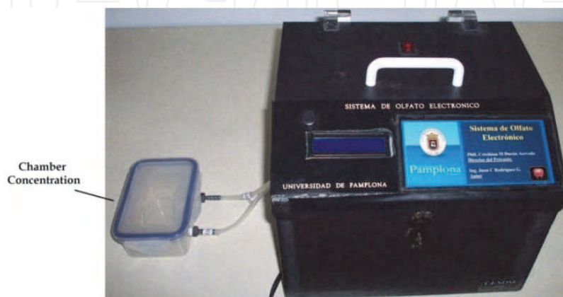
Fig. 6. Chamber of concentration, container for the different samples to be analyzed.
