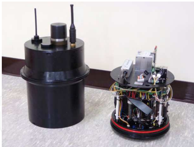
Fig. 3. Electronics system of P-SURO AUV.
