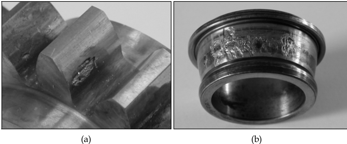
Fig. 2. The pitting wear: a) on a pinion gear, b) on a bearing race
