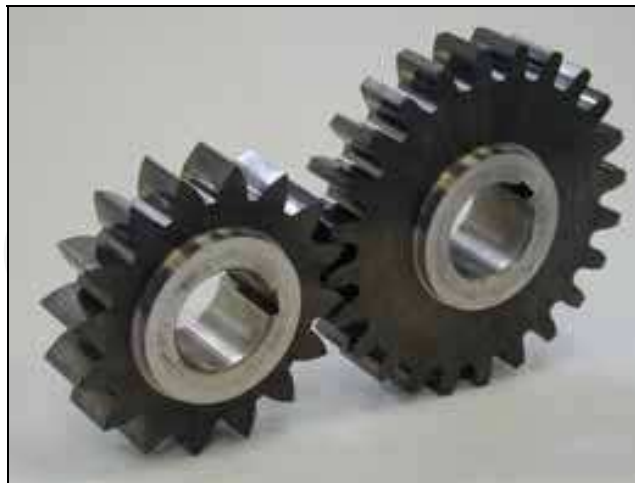
Fig. 12. Coated test gears used for testing scuffing - type A
