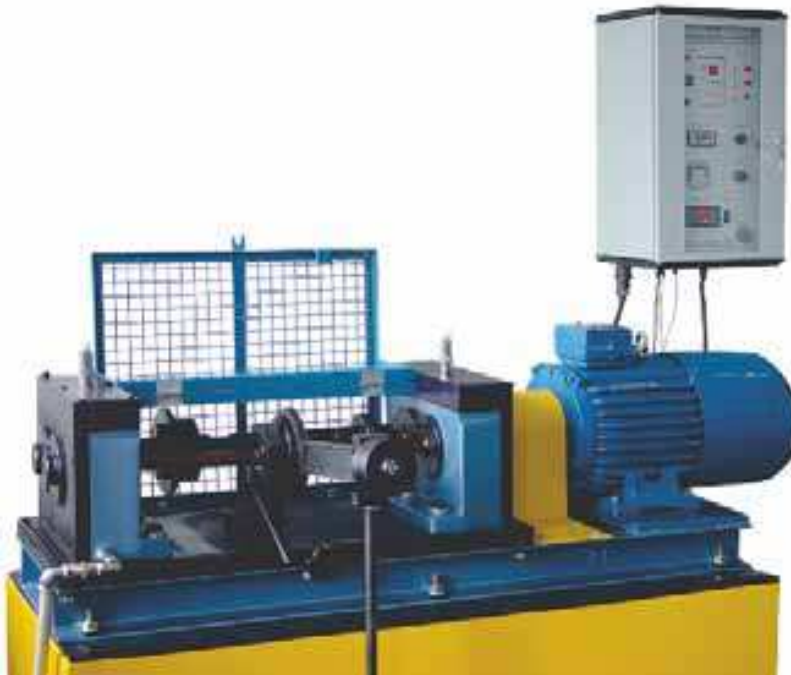
Fig. 17. T-12U Universal Back-to-back Gear Test Rig
