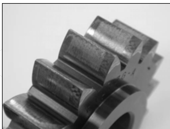
Fig. 1. A typical scuffing wear of gear teeth
