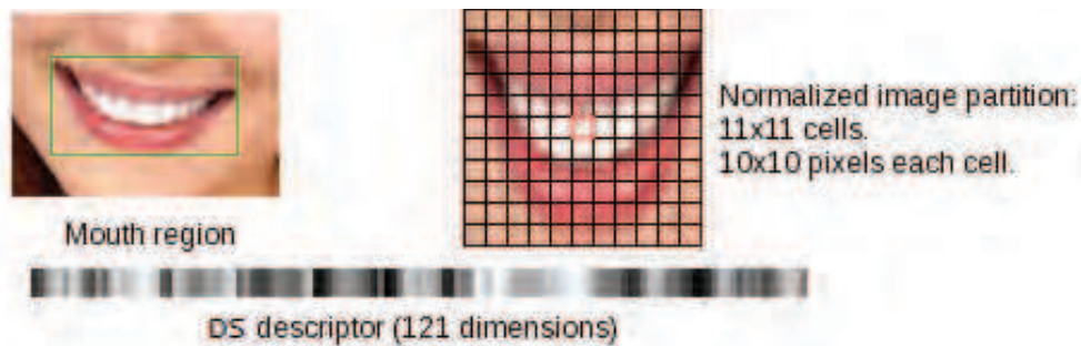
Fig. 5. DS Descriptor example using a 11x11 partition. The barcode-like vector represents all comparisons between each cell and the central patch. In this case, only the center patch will be considered to obtain our descriptor.
