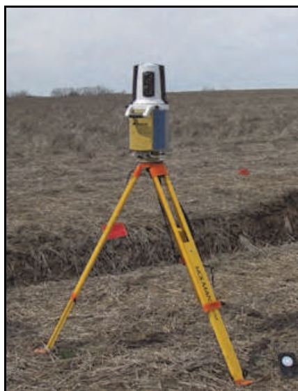
Fig. 1. Ground-based LiDAR utilized for gully formation and evolution studies in agricultural croplands.
