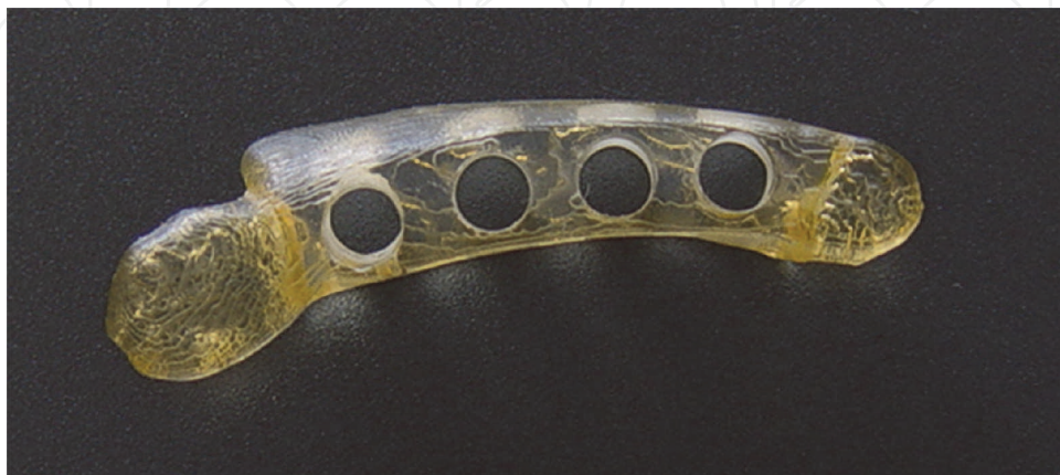
Fig. 6. Fabrication of the guide by stereolithography machine.
