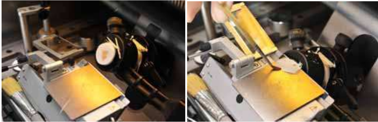
Fig. 5. Several 3-4 \mu\text{m} thick sections are cut after the tissue block is well cut in to expose flatly its entire surface.
