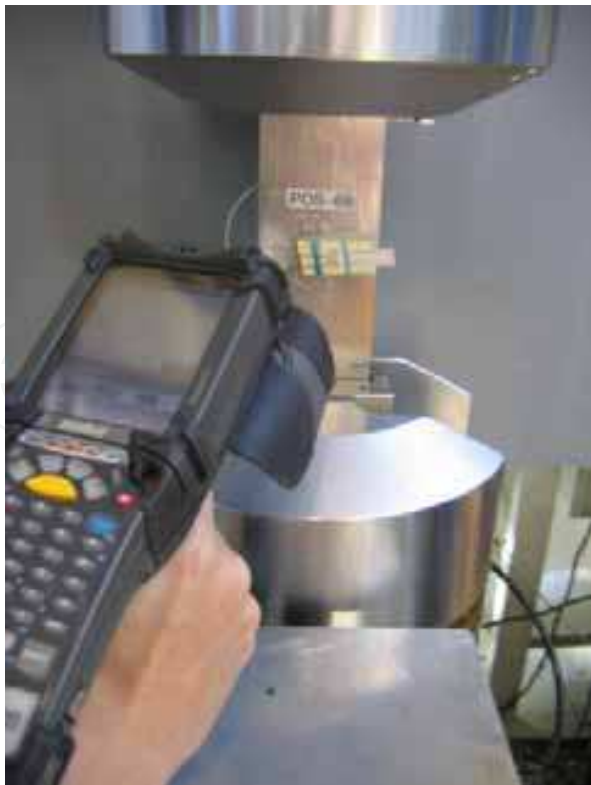
Fig. 20. Illustration of an RFID-based crack detection approach.
