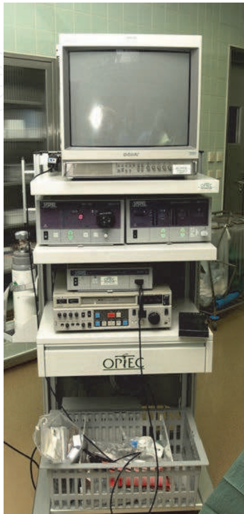
Fig. 8. The video monitor, recorder and light source are stacked on a portable cart.
