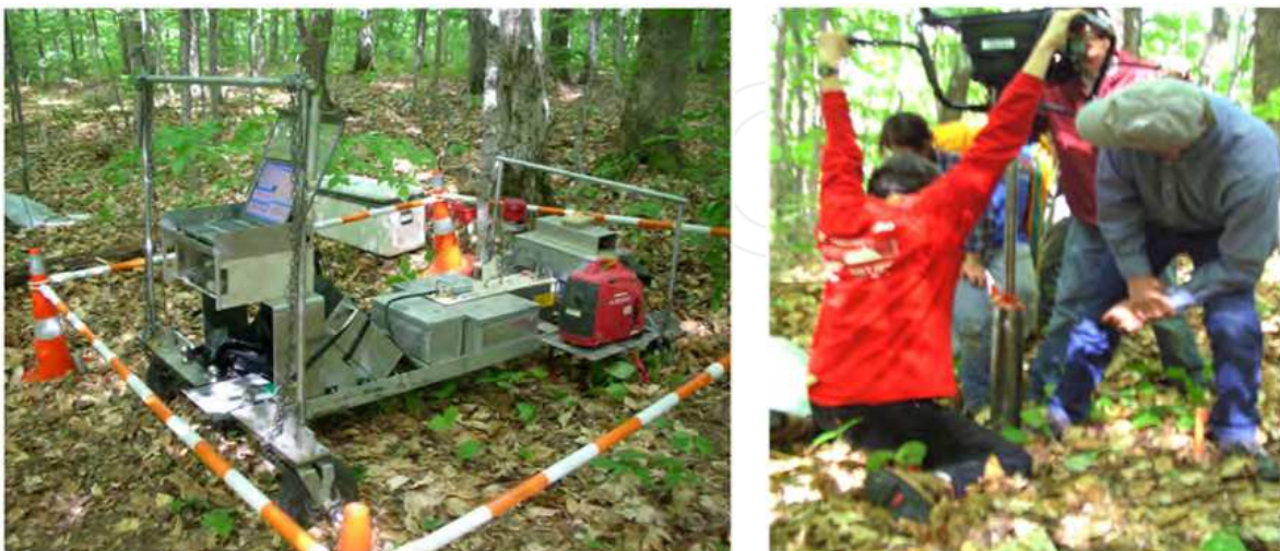
Fig. 13. On the left an INS set up measures the forest soil. On the right, a mechanized coring tool is used to sample soil from the forest floor. Many cores were abandoned because of the belowground rocks.
