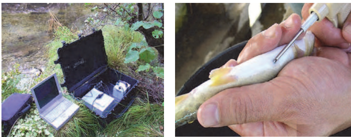
Fig. 5. PIT equipment (battery-pack and multi-point decoder- MPD) unit and PIT tagging procedures.
