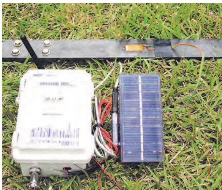
Fig. 6. Sensor node with a solar panel
