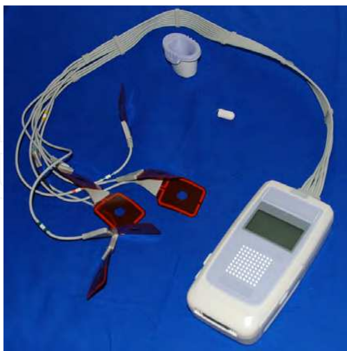
Fig. 3. Recording unit with the receiving electrodes. The videocapsule itself, as well as the initial cradle are pictured above.
