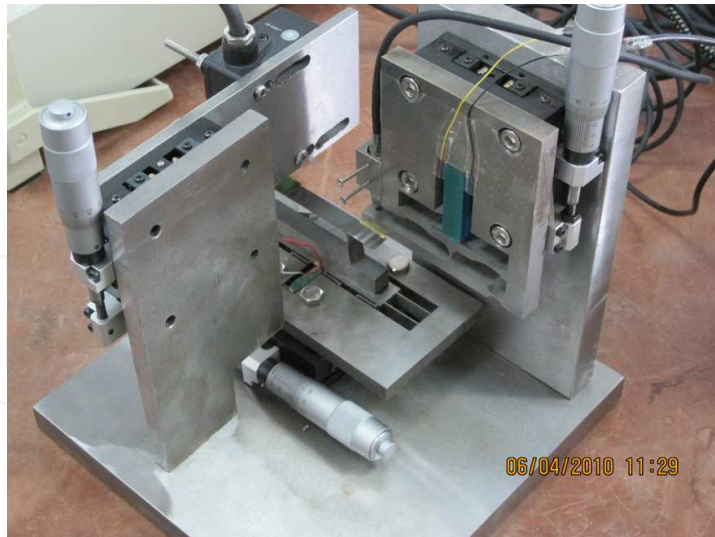
Fig. 21. Prototype of designed indentation device
