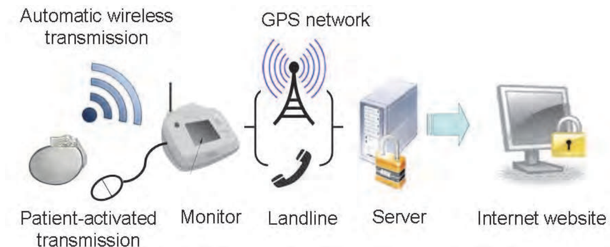
Fig. 1. Components of remote monitoring system. Systems differ regarding data transfer, which may require patient's active involvement or is performed wirelessly from the implanted device to a patient monitor. Data from the patient monitor is sent to a central database using either an analogue phone landline or via GSM network. The data are accessible to the clinical staff on a secure Internet site.
