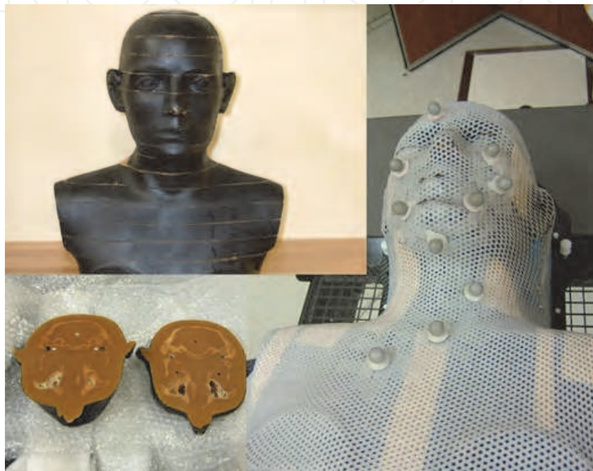
Fig. 2. A phantom for fundamental experiment. A sphere ball of 5mm diameter was inserted to phantom. IR markers were put on the phantom.
