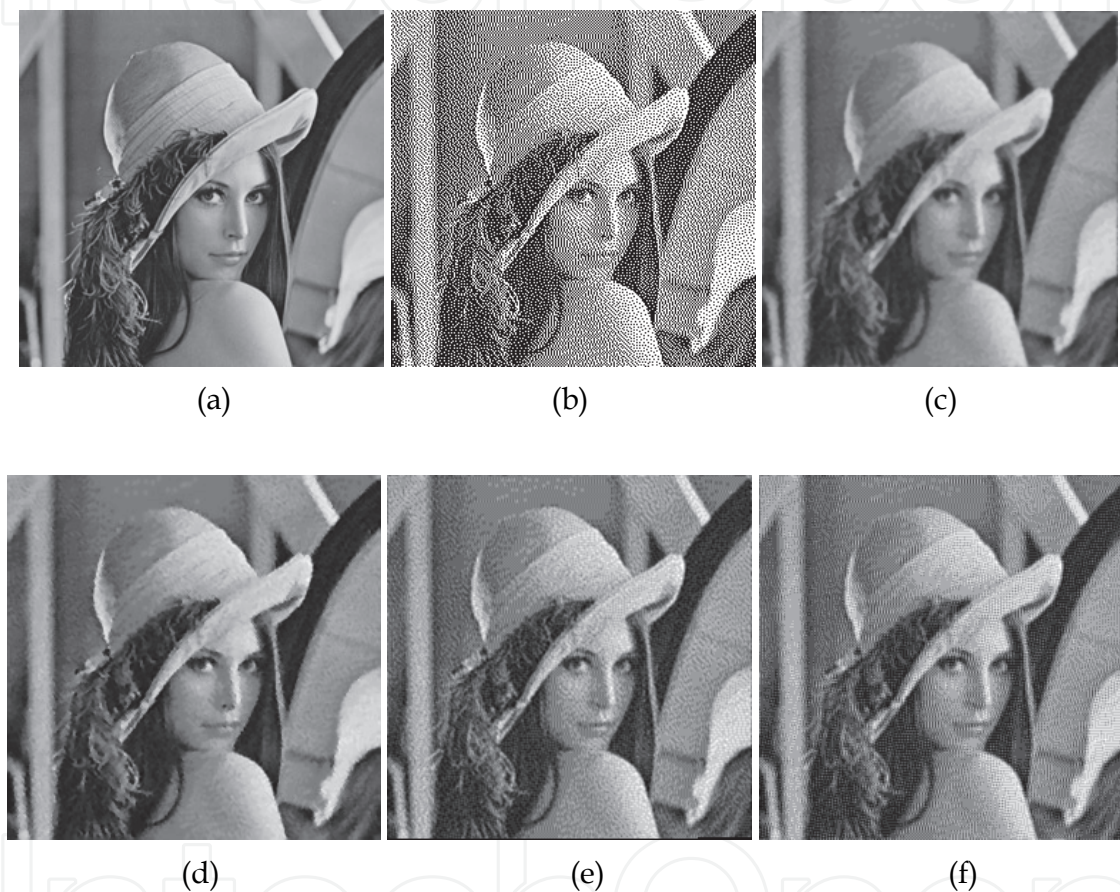
Fig. 10. (a) the 256-level standard image “Lena” with 256 \times 256 pixels, (b) the halftone image converted from the standard image (a) by the error diffusion using the Floyd-Steinberg’s kernel, (c) the restored image due to the GSS when \kappa=2.5 and D=0 (d) the restored image using the GSS when \kappa=2.5 and D=25 , (e) the restored image obtained by the Gaussian filter, (f) the restored image obtained by the average filter.
