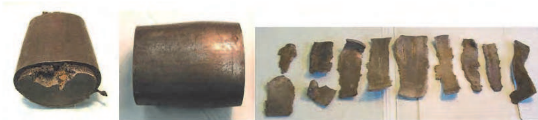
Fig. 4. Explosion-driven deformation of steel-cased PBXN-109 charges. The deformation results from the detonation of a layer of plastic explosive that partially surrounds the PBXN-109 charges (see Fig. 5). Results are shown for plastic explosive layer thicknesses of 3 mm (left), 4 mm (middle) and 5 mm (right).
