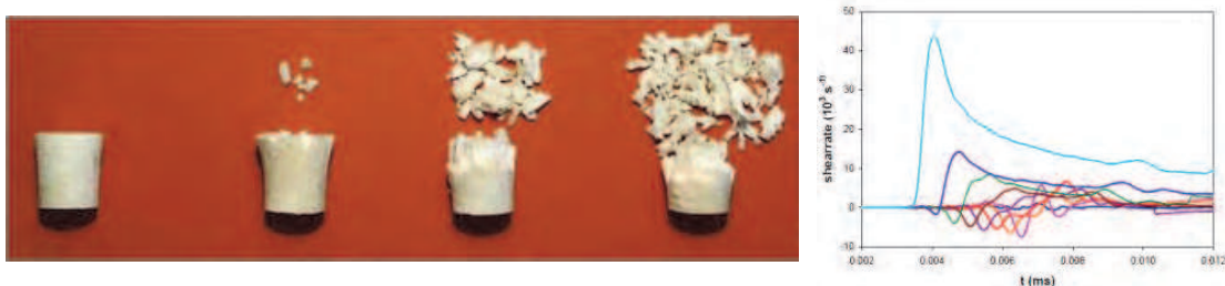
Fig. 6. Left: Permanent deformation and fracture of a PBX containing 80% HMX at 91, 110, 121, and 154 \text{m}\cdot\text{s}^{-1} impact velocity in a friability test. Right: The evolution of shear rate at various radial distances from the sample in the friability test and near the explosive/steel interface for PBXN-109 at 150 \text{m}\cdot\text{s}^{-1} impact velocity. The maximum shear rate develops near the outer radius.
