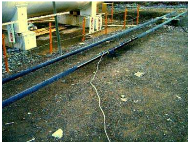
Fig. 4. Test to evaluate of equivalent thermal conductivity in the thermal insulated tubing using by pulsed heating carried at Yubari CO 2 -ECBMR test field (Oct. 10, 2006) (see Yasunami et al., 2010)
