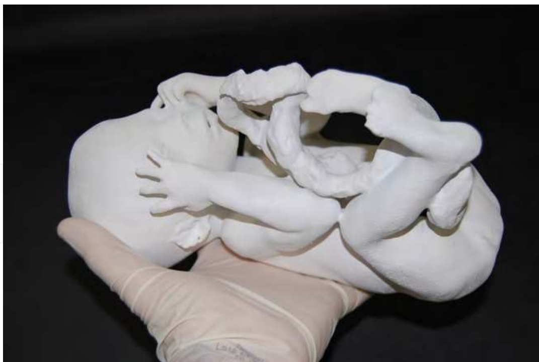
Fig. O. Physical model of 34 weeks fetus built on Z Corp 510 from Magnetic Resonance scan.
