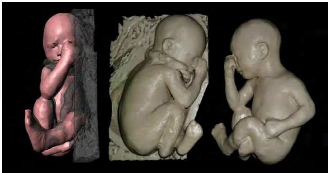
Fig. E. 32 weeks fetus built on Z Corp 510 from MRI files - on the left including the uterus and the umbilical cord and on the right only the body of the fetus.
