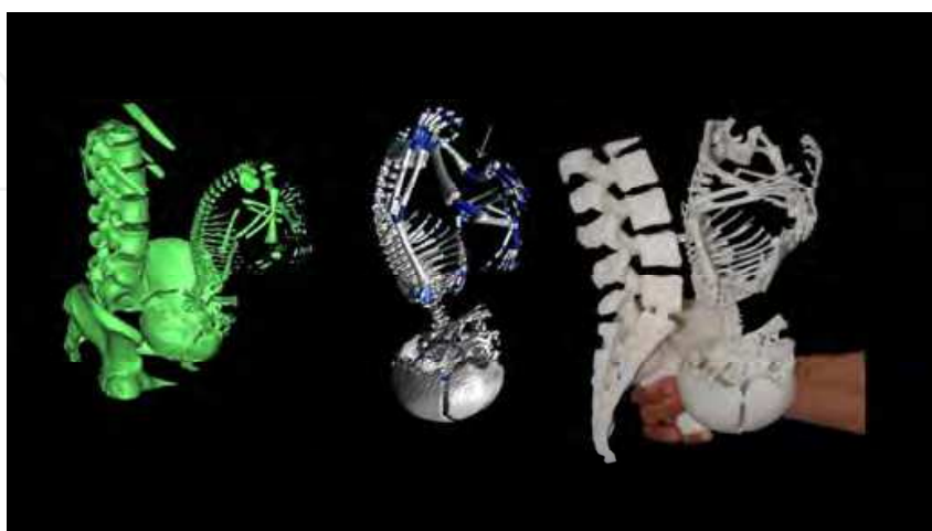
Fig. B. 34 weeks, 3D virtual and physical models of the skeleton of the fetus built on SLA (3D systems - Viper Si) from CT scan.
