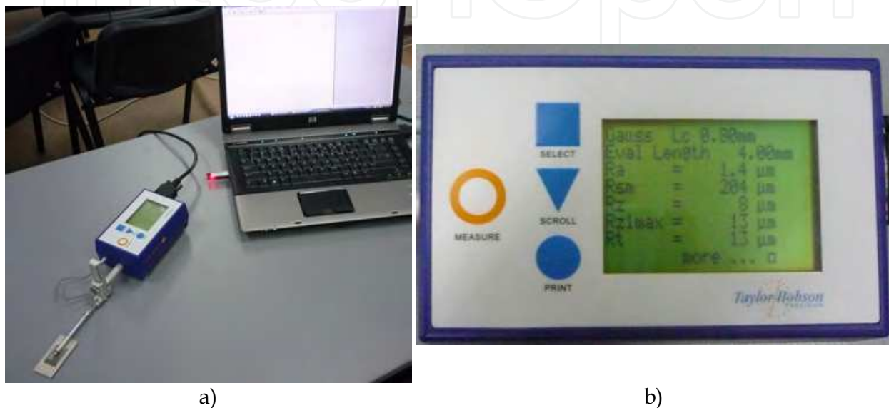
Fig. 32. The parameters calculated by “Surtronic 25”
