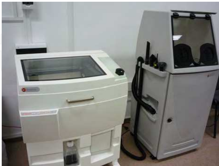
Fig. 6. Z 310 Plus printer and its depowdering station (compressed air system and vacuum suction system) - Transilvania University of Brasov
