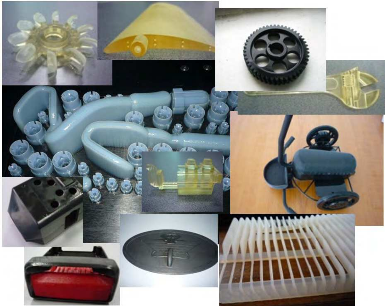
Fig. 29. Products obtained by “polyjet” printing (EDEN 350), Transilvania University of Brasov
