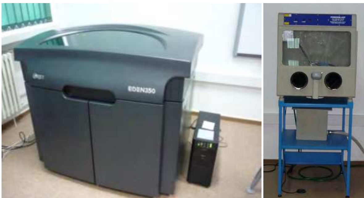
Fig. 8. EDEN 350 printer and its water jet recycle station - Transilvania University of Brasov
