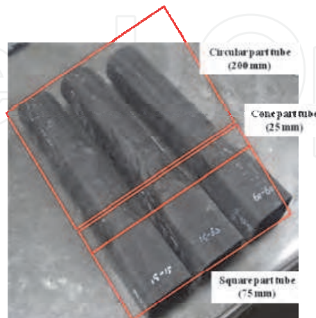
Fig. 13. Fabricated carbon braided FRP tubes with a novel three-phases geometry: circular part of 200mm, cone part of 25mm and square part of 75mm
