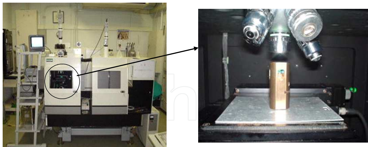
Fig. 5. Schematic picture of diamond anvil cell set upped with a Raman spectrophotometer (JASCO NR-1800).
