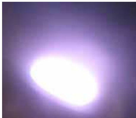
Fig. 8. Photograph of the typical glow from ZnO target when sputtering.
